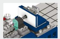
The company's EOL tester evaluates the functionality and assembly ability of key electric vehicle parts such as the EDU, gearbox and HEV. Various tests carried out automatically on this test bench are for the verification and testing of safety-related items inside the motor of EV/HEVs
